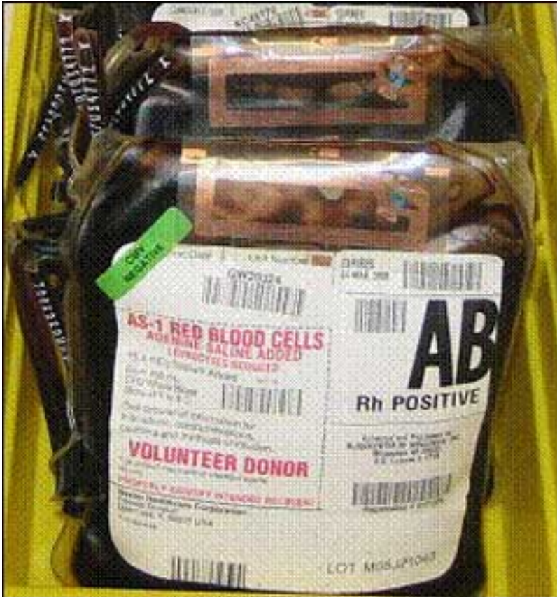
During the project's first phase, researchers used blood bags fitted with adhesive 13.56 MHz passive RFID tags.
