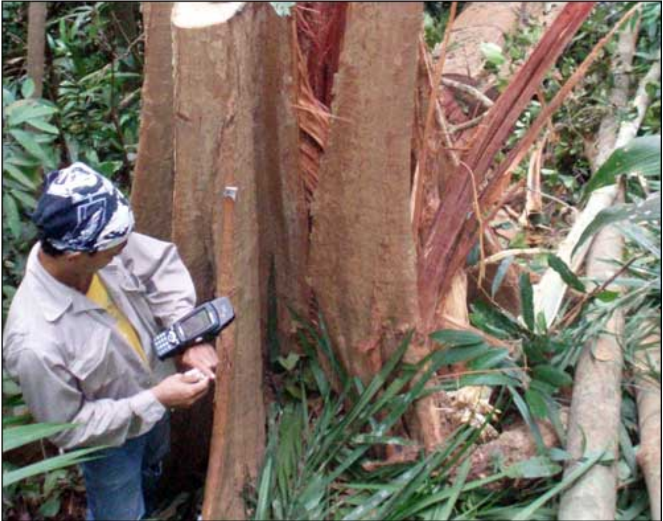
A forestry department employee reads the RFID tags of a felled tree.
