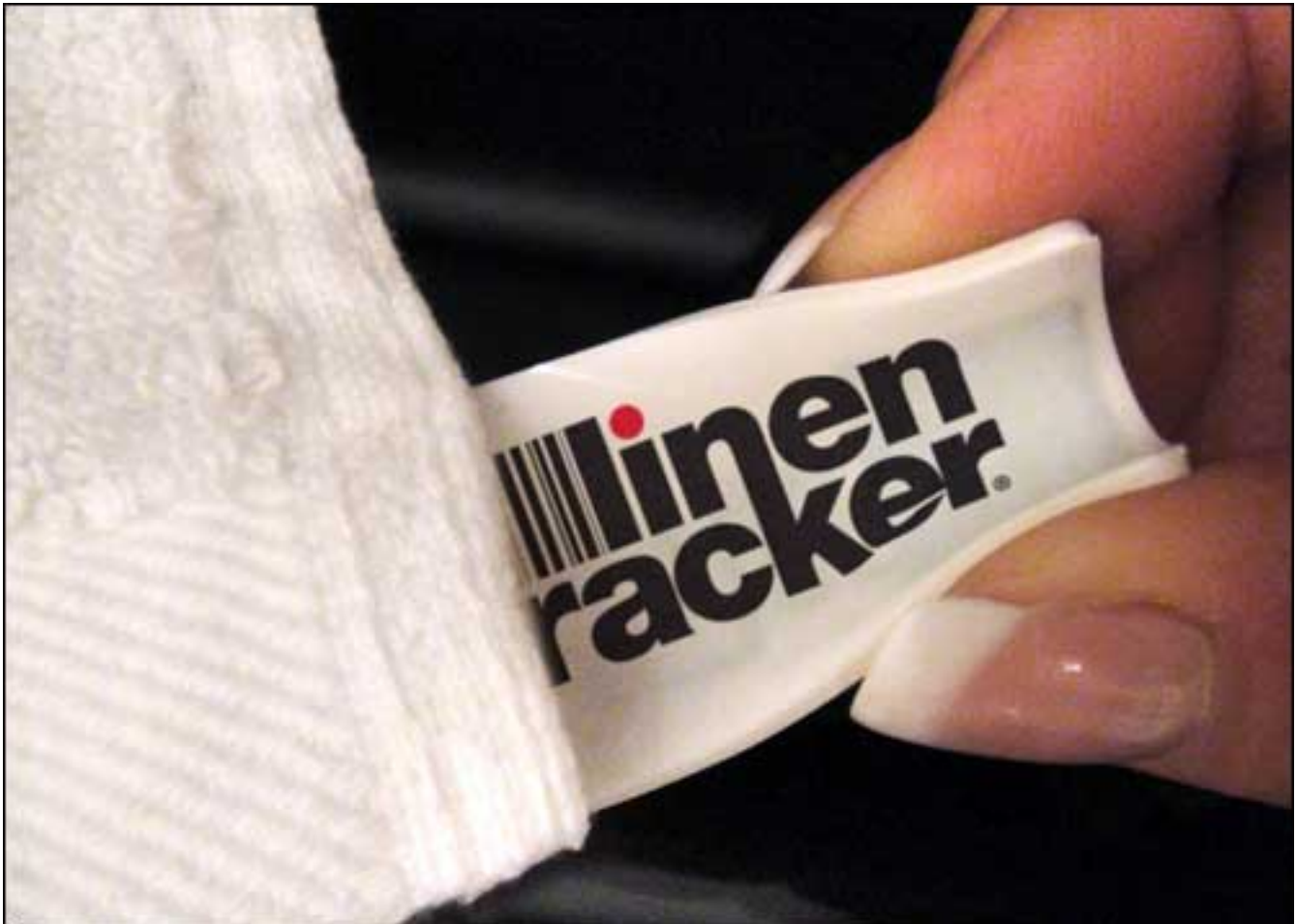
LinenTracker's RFID tag contains an EPC Gen 2 inlay from Alien Technology.
