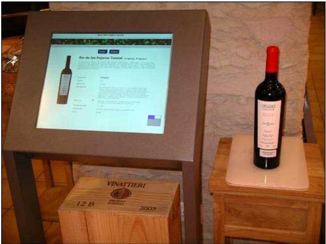
When a customer picks up a tagged bottle and sets it on a table fitted with a reader antenna, the kiosk's screen displays information about that particular wine.
