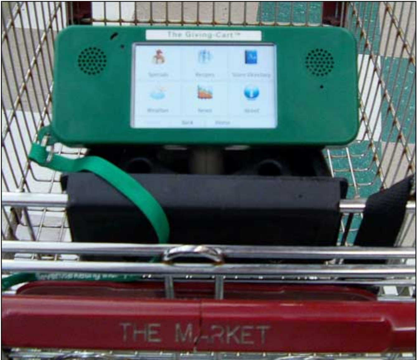
The Giving Cart mobile unit has a built-in RFID tag to identify a shopper's location within a store.
