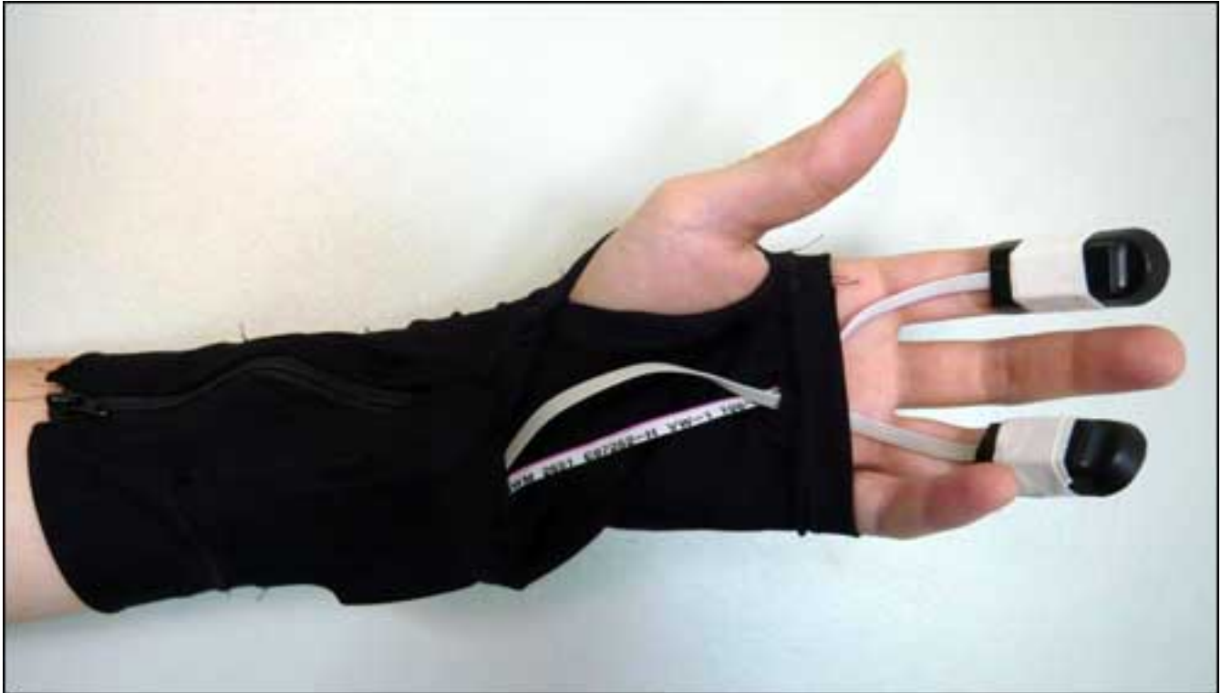
Each glove contained a Ubisense active RFID tag, as well as wireless sensors that tracked the electrical conductivity of the wearer's skin, as well as pulse.
