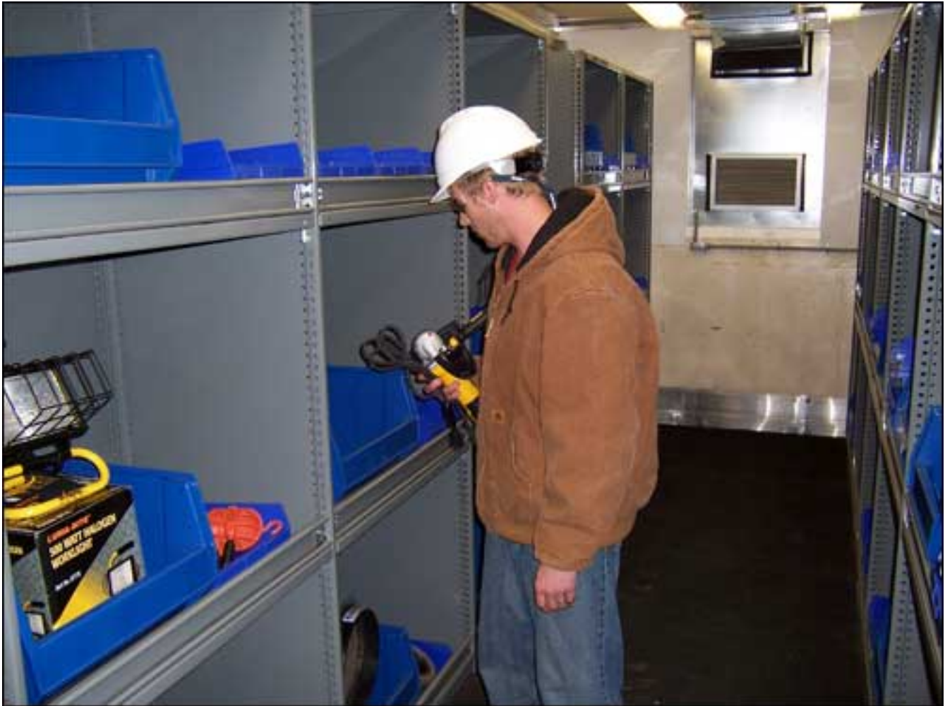
An employee selects the tools required for a specific job, then walks out of the trailer, passing through a portal so that his badge ID and the tool tag IDs can be read by an RFID interrogator.
