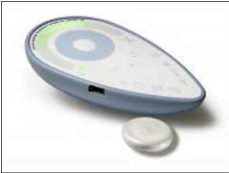
The system uses a 125 kHz RFID tag and sensor, in conjunction with a handheld RFID interrogator.
