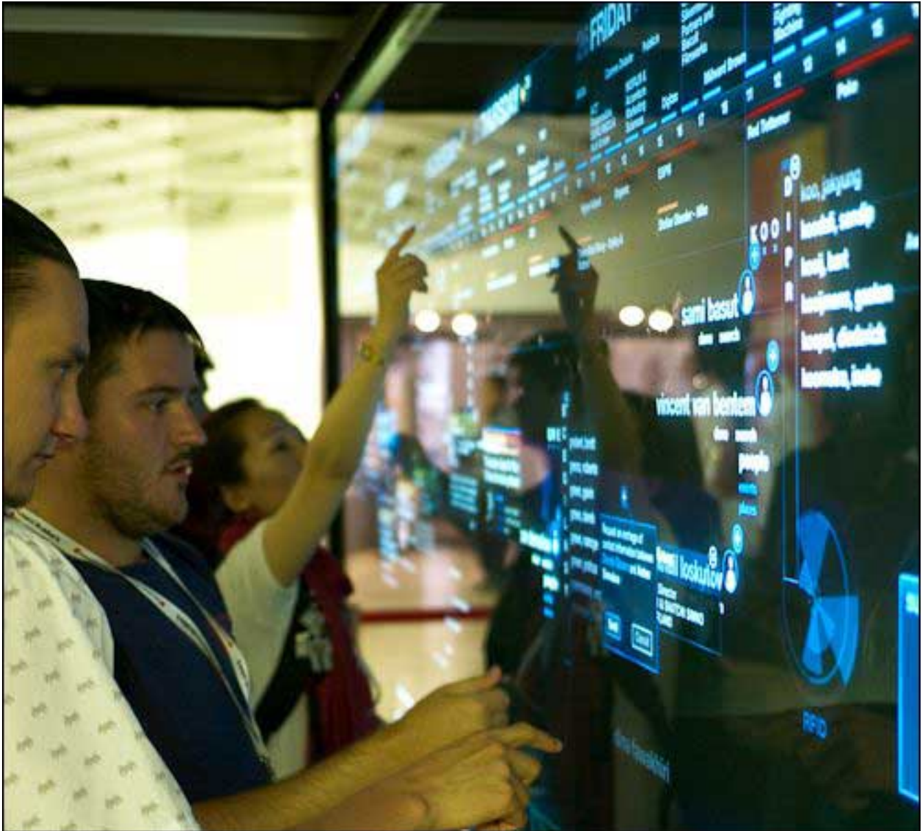
Standing at the Touchwall, users identify themselves via RFID, then use their fingers to select and drag text and objects.
