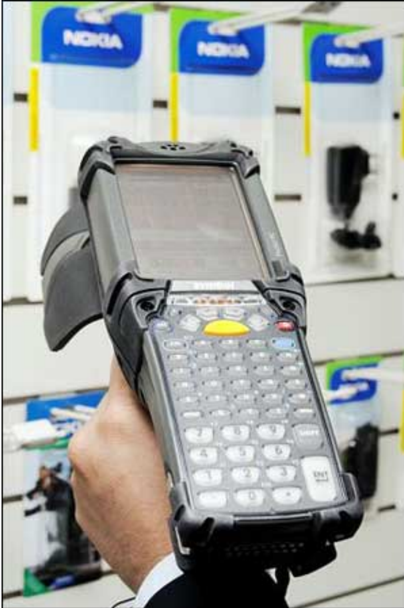
The Future Communications staff use a Motorola handheld reader to inventory goods on the sales floor.
