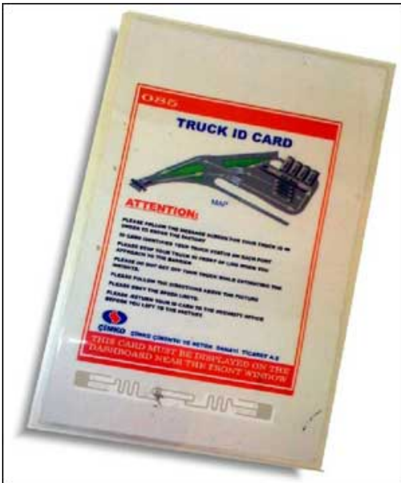
A Cimko truck ID card contains an Alien Technology EPC Gen 2 RFID tag.
