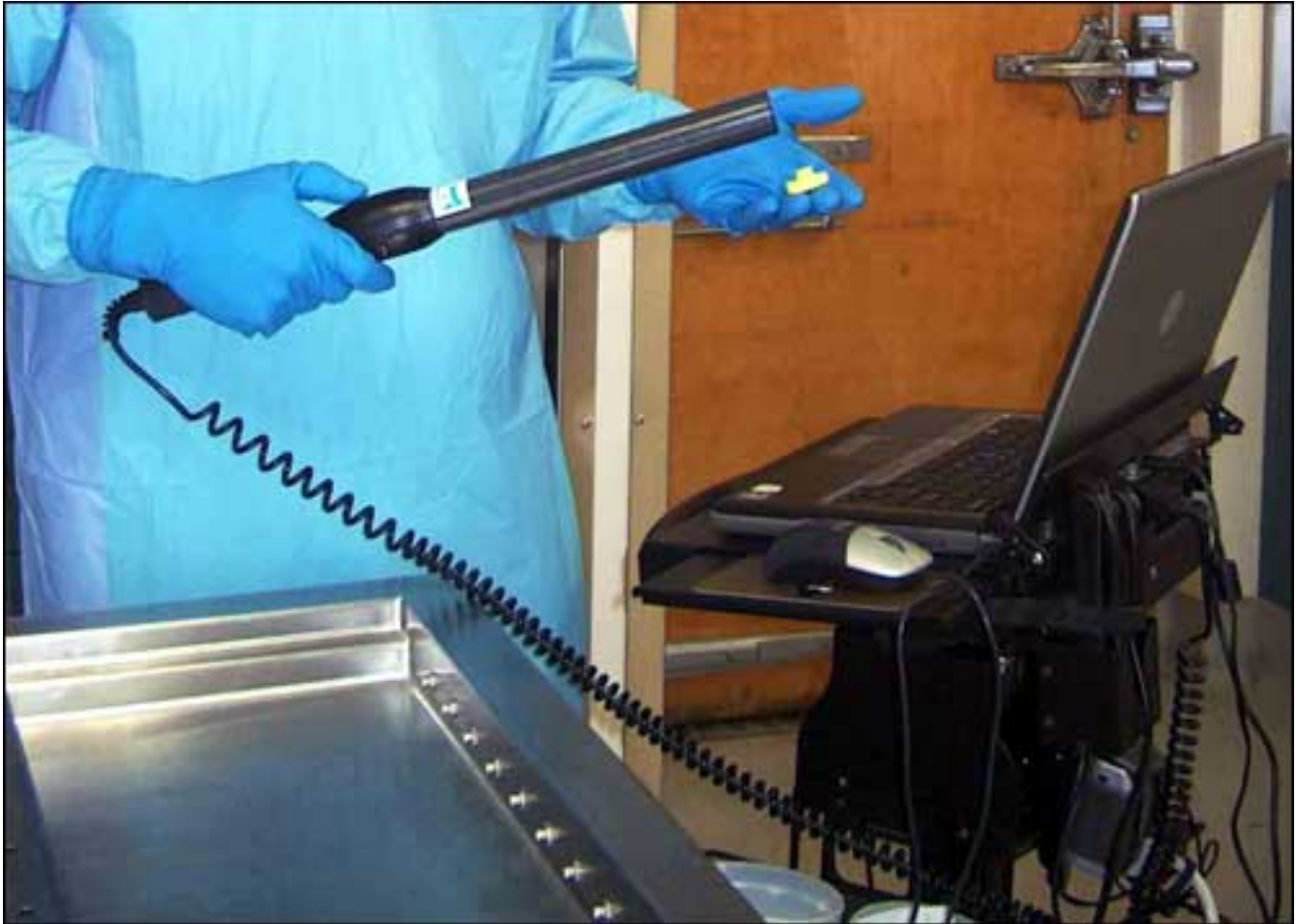
To read the tags, lab workers use a wand-shaped handheld RFID reader.
