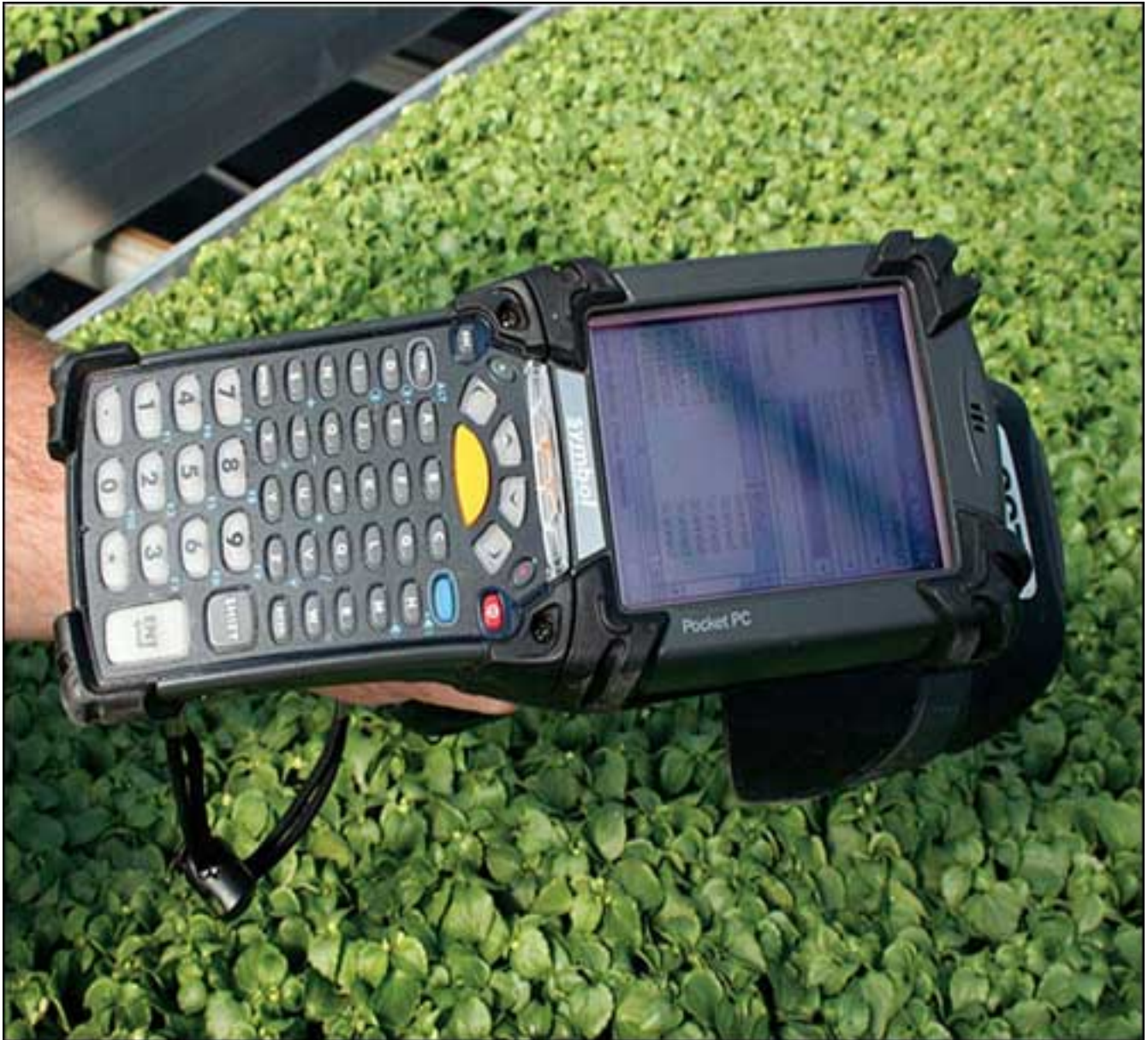
Handheld interrogator for reading tray tags
