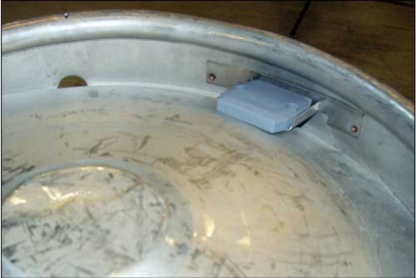
Each keg is fitted with an EPC Gen 2 passive UHF tag made by Confidex.
