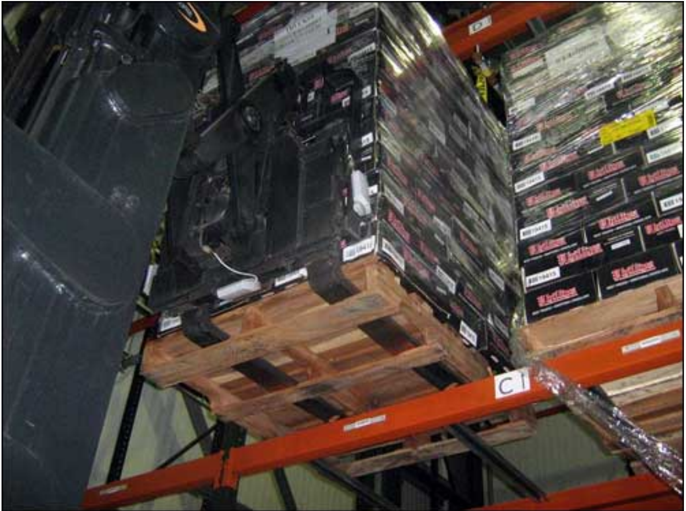
A forklift's RFID reader captures the rack tag's ID number, thereby identifying the pallet's exact storage location.
