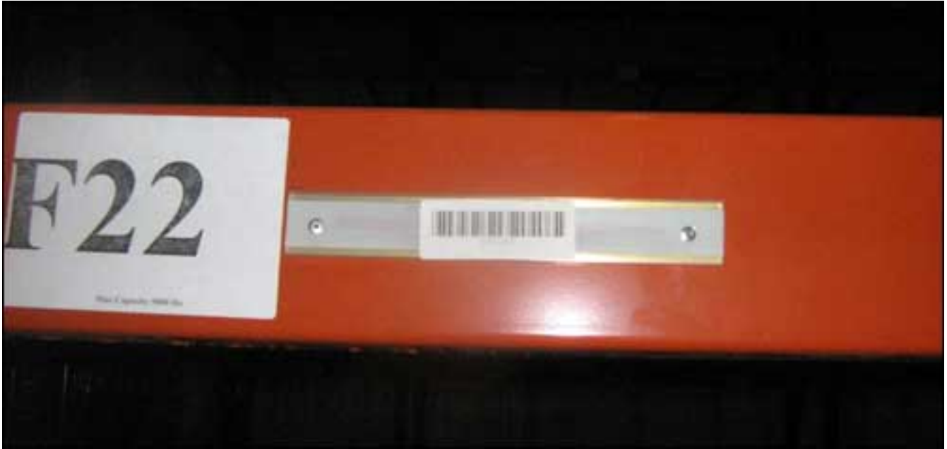
Each of about 1,600 rack locations in cold storage is marked with an RFID tag.
