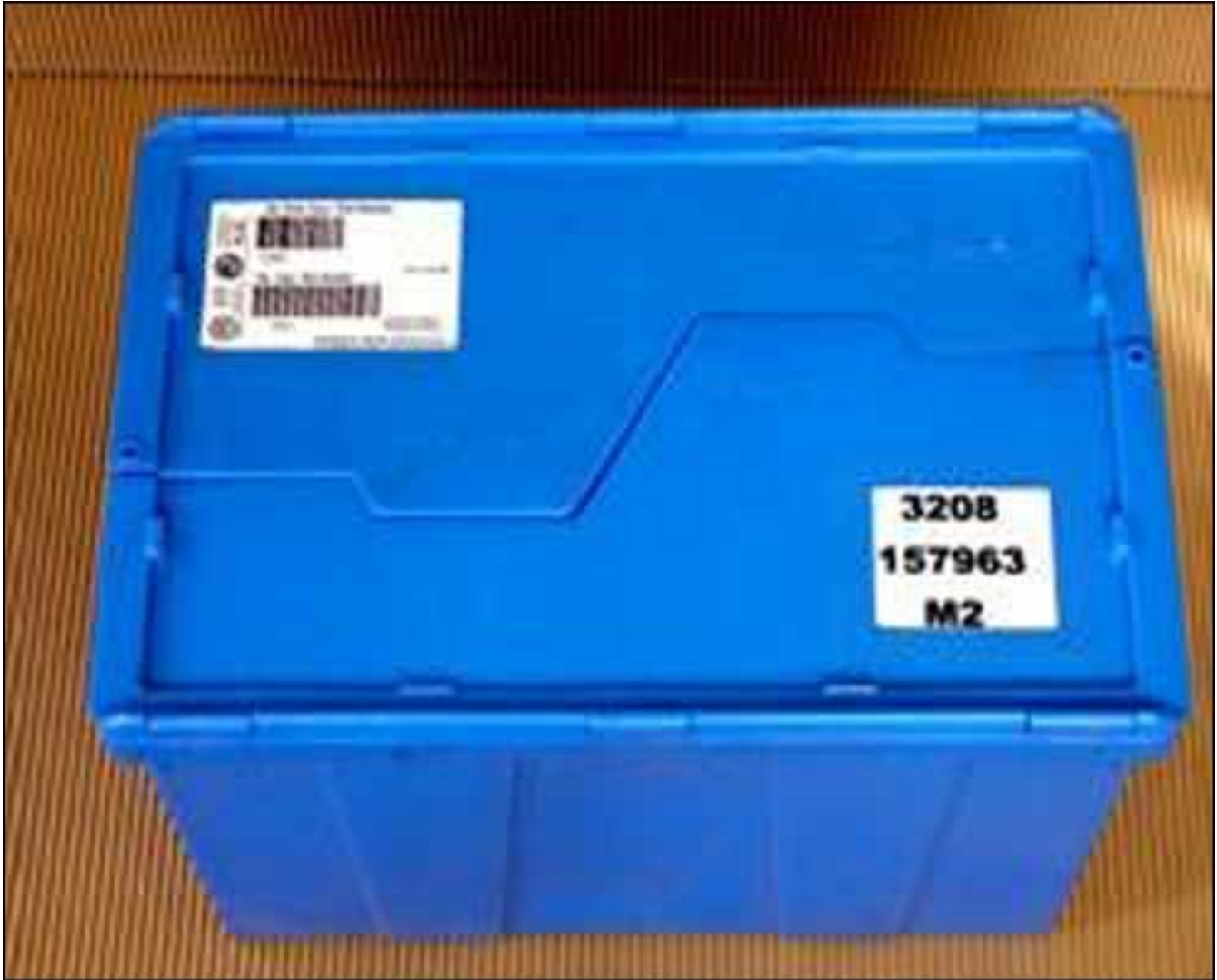
Each of VW's plastic containers, used for shipping parts, is fitted with a bar-coded label containing an EPC Gen 2 RFID tag.
