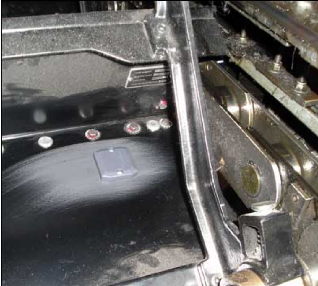
The underside of each escalator step is fitted with an Ironside EPC Gen 2 RFID tag from Confidex.
