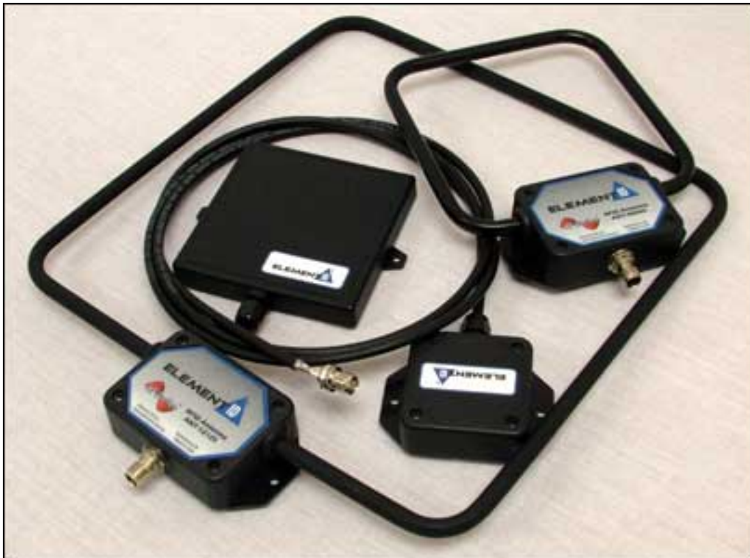
Element ID's interrogators work with a variety of external antennas.
