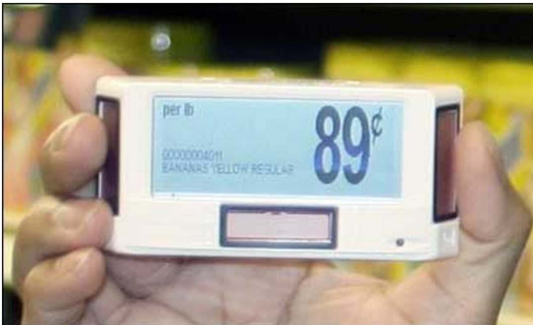
Altierre's electronic shelf label contains a 2.4 GHz RFID tag and an LCD display.
