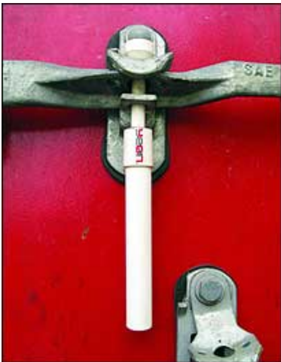
To seal a container door, the Yeon YTE-100's bolt locks onto the device's body. If the bolt is cut or removed, its RFID chip ceases to function.
