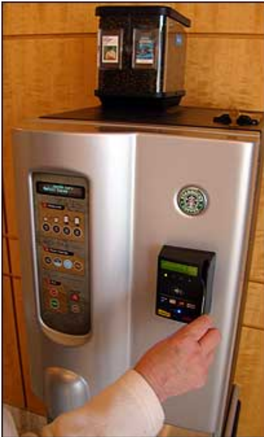
The Starbucks Interactive Cup brewing machine will accept RFID-enabled payment cards, as well as magnetic-stripe cards.
