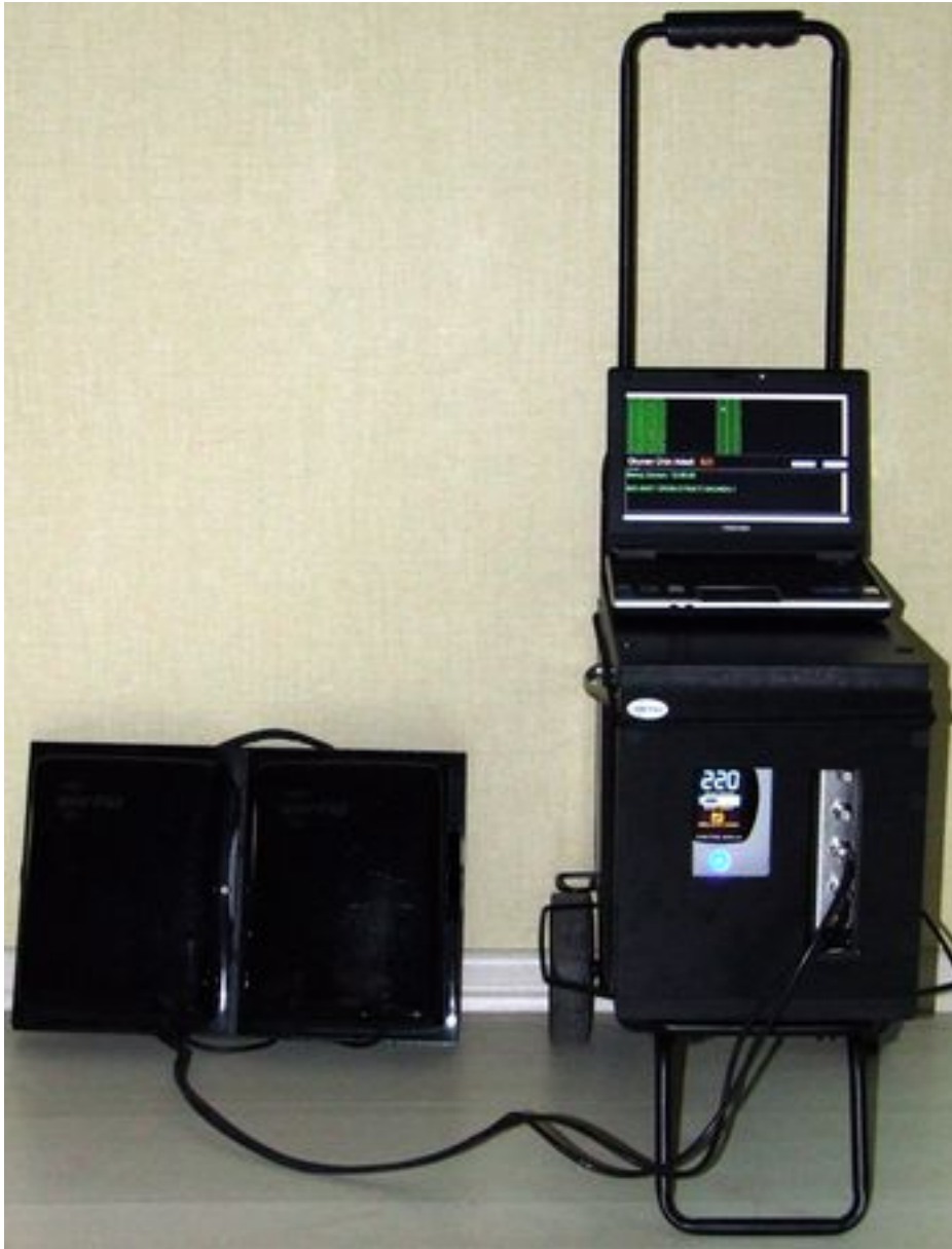
To take inventory inside Eren Holding's stores, one employee wheels a mobile RFID interrogator through the aisles, while another carries the interrogator's antenna.
