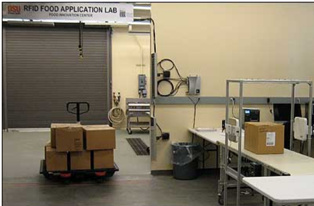
At OSU's RFID Food Application Lab, a portal and a variable-speed conveyor fitted with fixed RFID interrogators.
