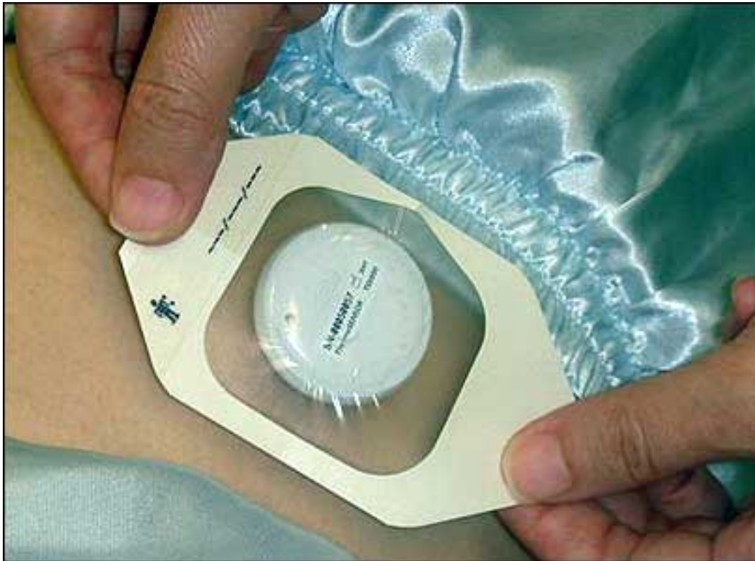
The ThermoSensor tag is taped to a patient's abdomen to monitor body temperature.
