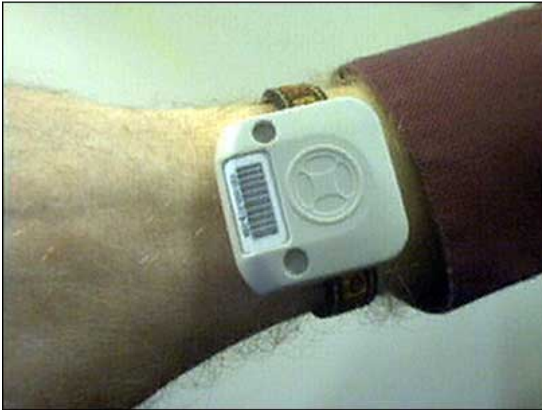
At the Shady Palms assisted-living facility, participating residents wore a battery-powered RFID tag on their wrists.
