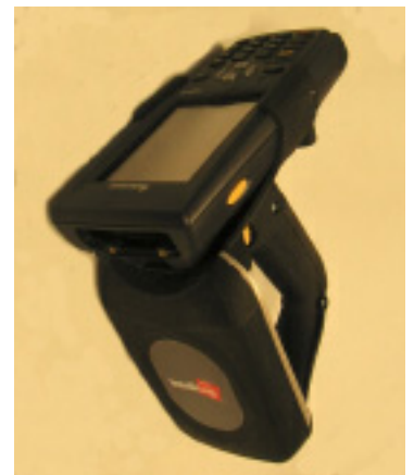
The IP3 grip reader and 700 Series handheld computer
