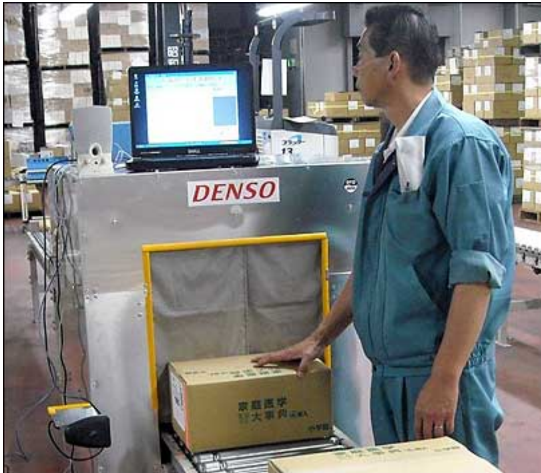
To fill an order from a retailer, Shogakukan packs the requested quantity in a carton and passes it through an RFID reader tunnel, thereby creating an electronic record of which books were shipped.
