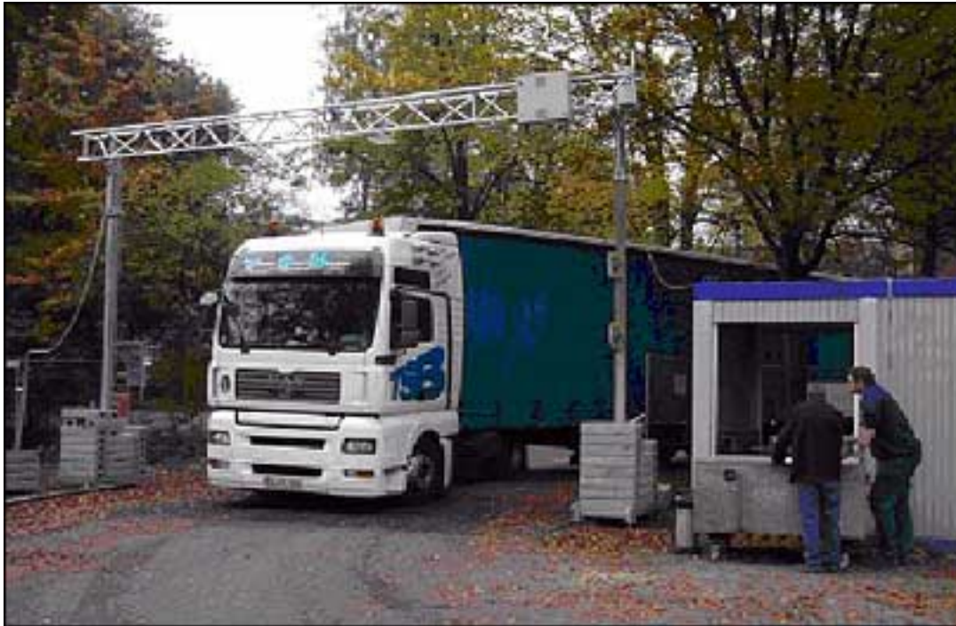
A truck carrying tagged facade elements passes an RFID gate.
