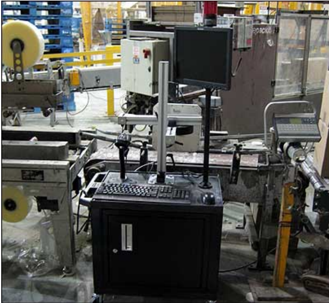
Normerica workers wheel an RFID-enabled cart to a station where Wal-Mart-destined products are being packed, thereby reducing the cost of installing an RFID reader at each conveyor.
