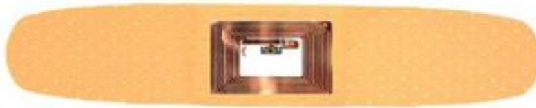
An adhesive skin patch (above) contains a passive 13.56 MHz RFID tag wired to a battery-powered noninvasive sensor (below) that measures a person's glucose level.
