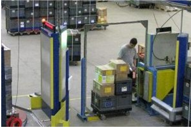
To track the movements of pallets and dollies at its facilities, Manor uses transition portals.
