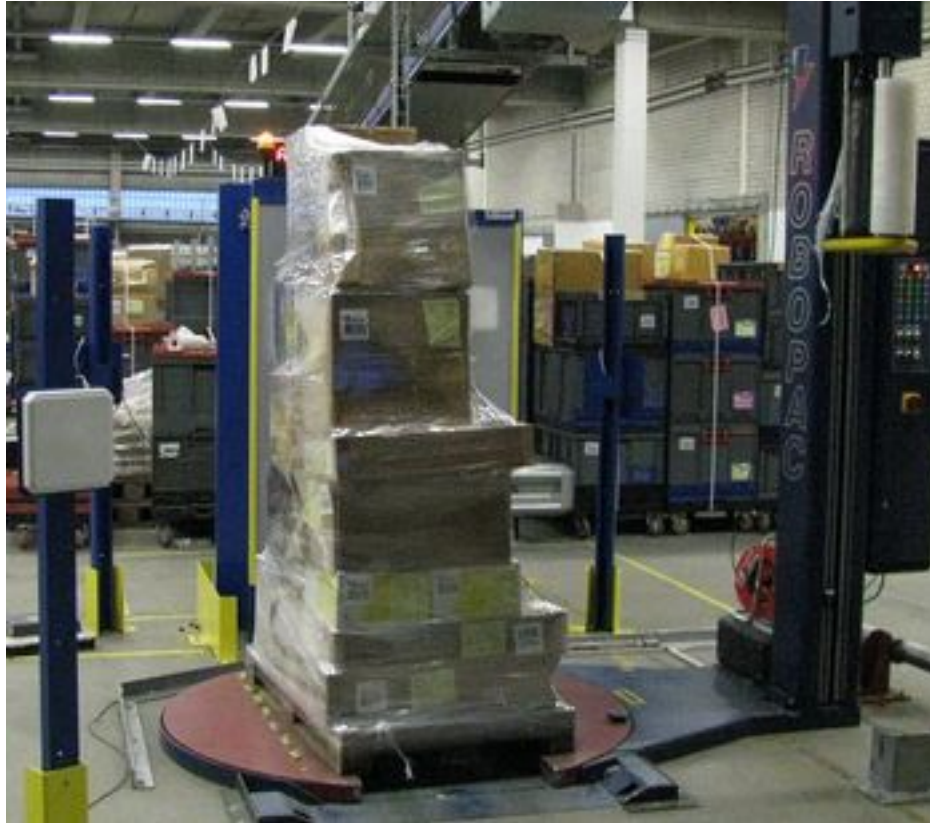
At a Manor's DC in Möhlin, a pallet's contents is recorded automatically by an RFID reader installed at the stretch-wrapping station.
