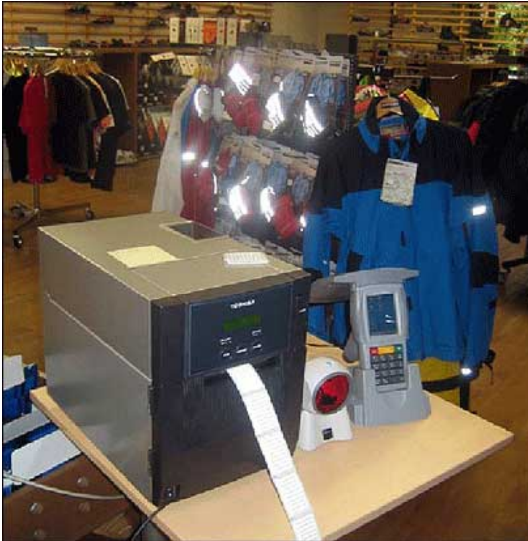
The store's RFID station includes a printer-encoder for generating RFID labels and a handheld interrogator for taking inventory of tagged goods.
