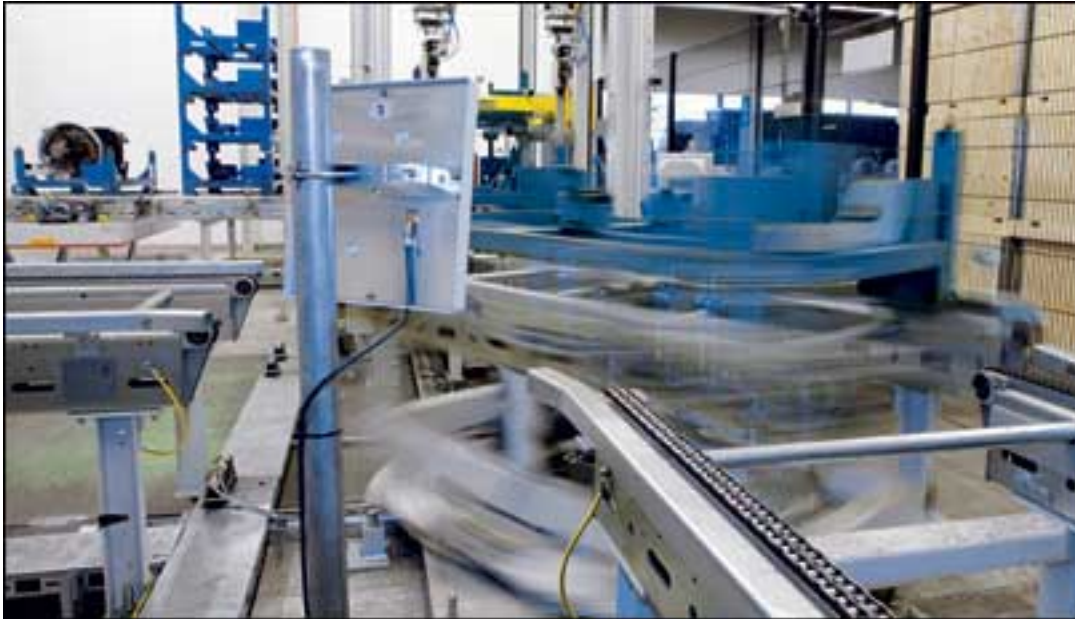
As a container moves along the conveyor track, an RFID reader identifies it.
