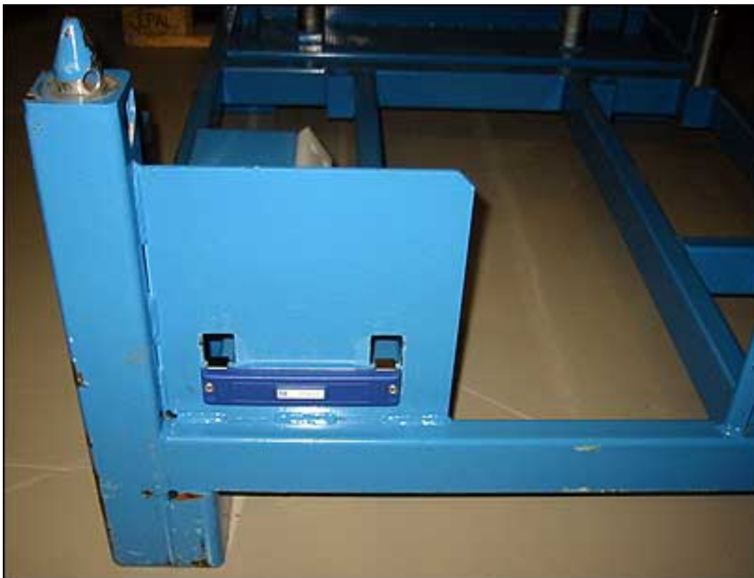
A passive UHF tag is attached to each container.
