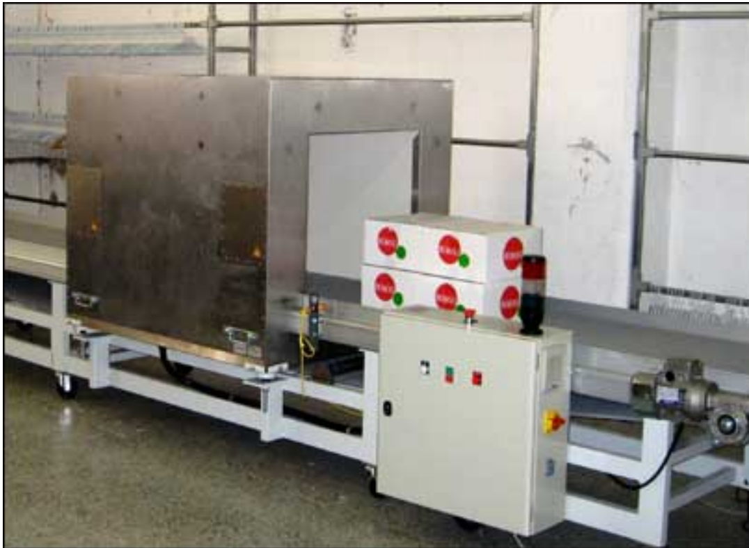
At the DC, cases of the tagged garments will be placed on a conveyor belt and moved through a Tagsys interrogator built into a tunnel form factor.
