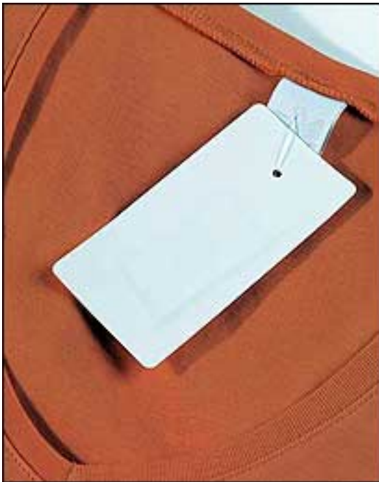
A hangtag, containing a UHF passive EPC Gen 2 inlay pre-encoded with an Electronic Product Code, will then be attached to each article of clothing.
