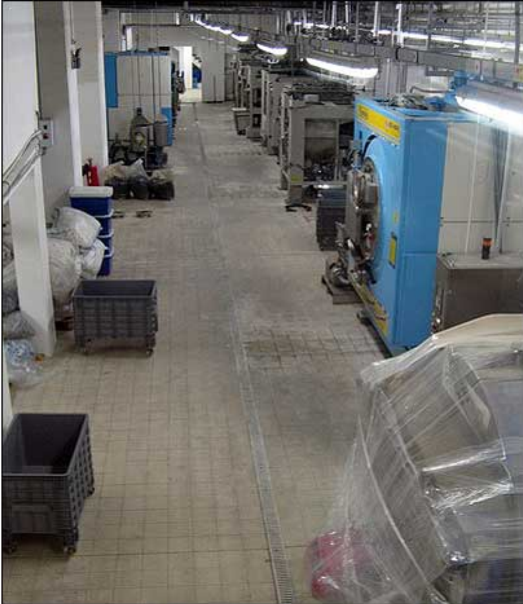
Gelal uses wheeled plastic totes, fitted with EPC Gen 2 tags, to track socks as they are transported from one production station, such as this dyeing room, to the next.
