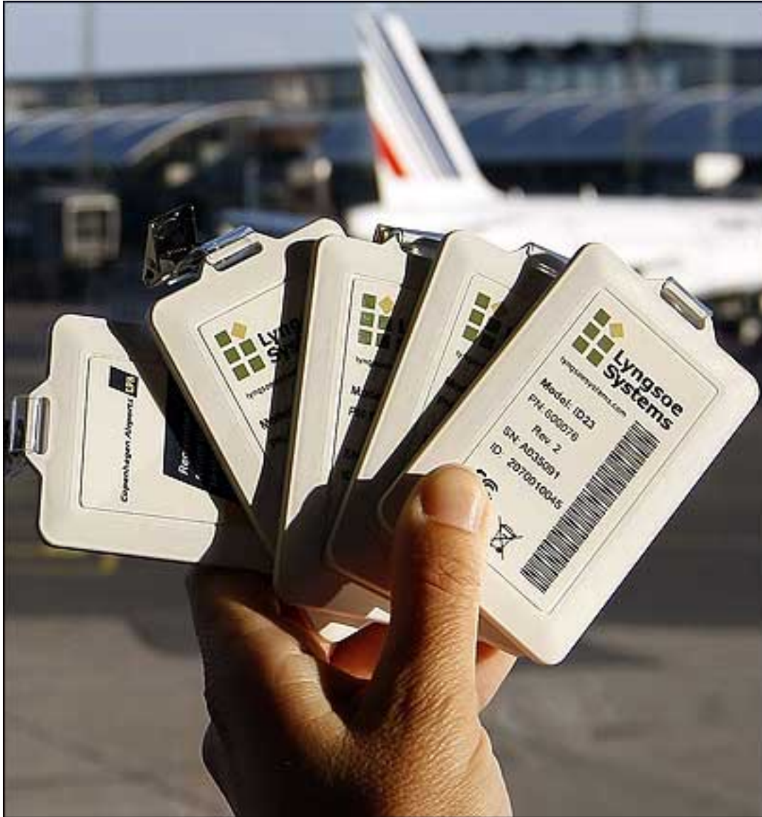
The Gatecaller project uses active 433.92 MHz to track the location of air passengers.
