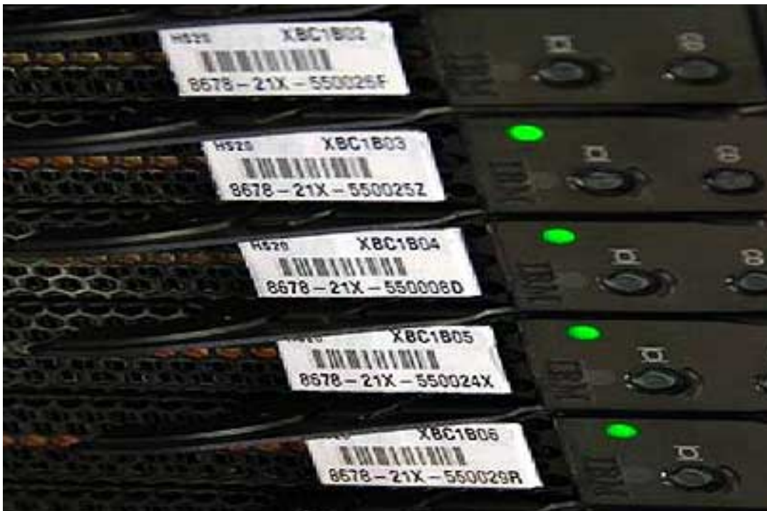
Omni-ID Prox tags are applied to blade servers.
