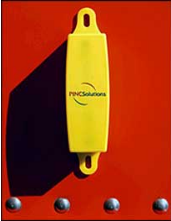
Each trailer is identified by an EPC Gen 2 passive RFID tag embedded in encased in a rugged housing and permanently mounted onto the trailer.
