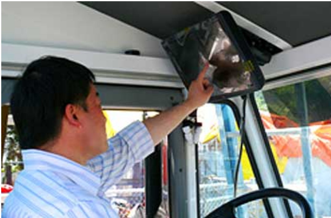
CPWM truck drivers can use a touch-screen computer to see a map of the yard, showing them where each trailer should be placed.
