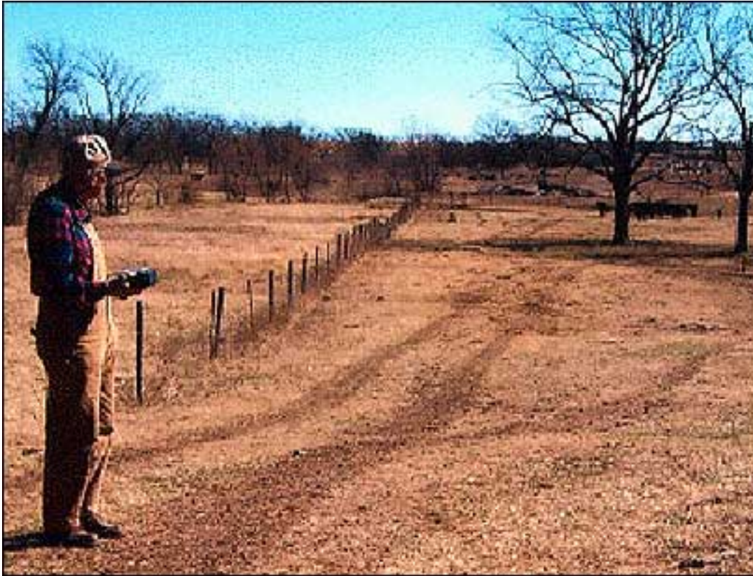
ZigBeef-tagged cattle can be read several hundred feet from a ZigBeef reader.
