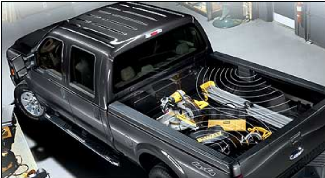
Each time the vehicle's engine starts, a built-in interrogator reads the tags of items placed in the bed or cargo hold.
