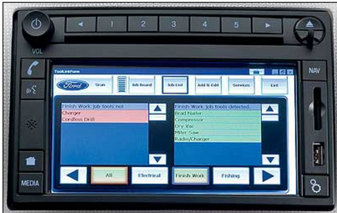
The vehicle's in-dash computer's screen can display a list of all tagged items onboard.
