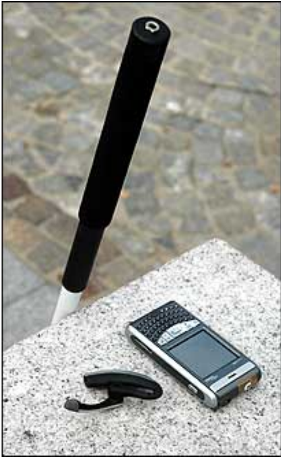
SESAMONET user components consist of a walking cane, earphone and PDA.
