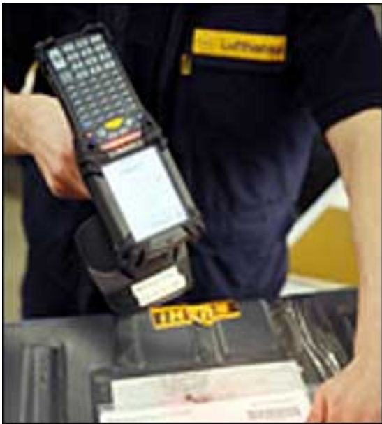
Lufthansa Technik is using handheld interrogators to read the tagged documents that accompany aircraft parts.
