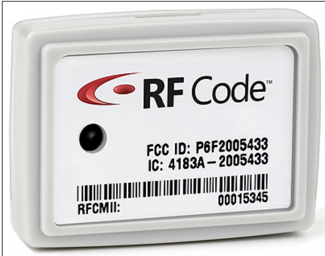
The M100-i tag contains a motion sensor that turns off the built-in IR receiver when the tag is stationary, reducing the tag's beacon rate.
