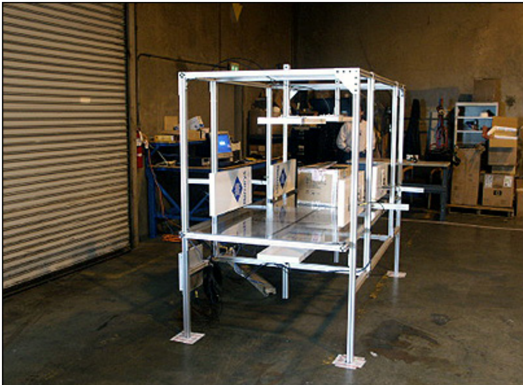
A readout station used to track items with RFID technology.
