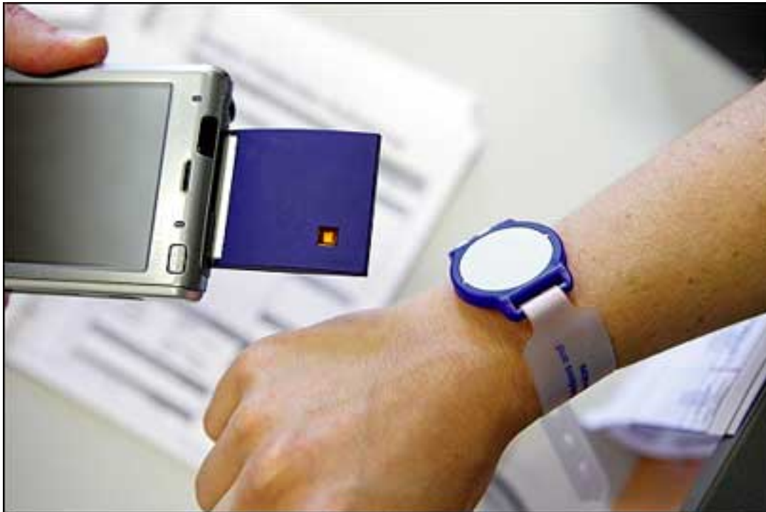
The system will be extended to blood bank supplies for about 1,000 patients, and works together with another system to identify patients via RFID-based wristbands.
